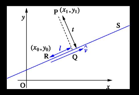
• Given:  $(x_0, y_0)$ ,  $(x_1, y_1)$  and  $\hat{v}$ , PQ  $\perp$  RS Q. Determine the location of Q, and determine t and l
