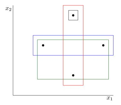
I drew in a few dichotomies in different colors. You should be able to complete the picture. Note that you cannot shatter a set of 4 points that are the corners of an axis-aligned rectangle, because then you won't be able to separate the two points on one diagonal from the two points on the other diagonal.
