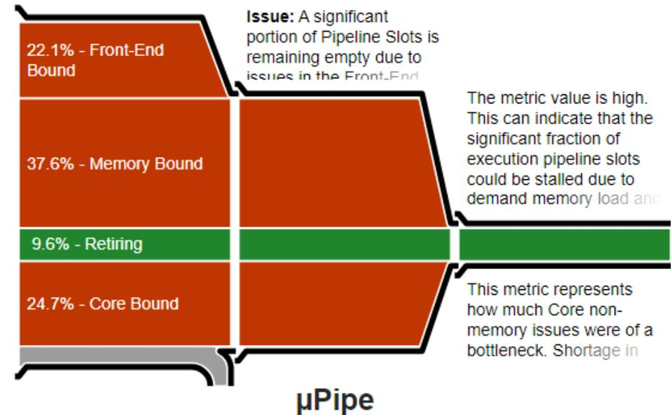
This diagram represents inefficiencies in CPU usage. Treat it as a pipe with an output flow equal to the "pipe efficiency" ratio: (Actual Instructions Retired)/(Maximum Possible [Instruction Retired](#)). If there are pipeline stalls decreasing the pipe efficiency, the pipe shape gets more narrow.
