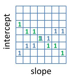
The middle of the cell with the highest number gives slope and intercept of a line with many points close by
